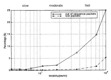
FIG. 17. Impact of mobility on out of order delivery and packet loss.
