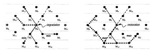
FIG. 10. (a) Degradation due to lack of resources. (b) Restorations through rerouting of a flow.
