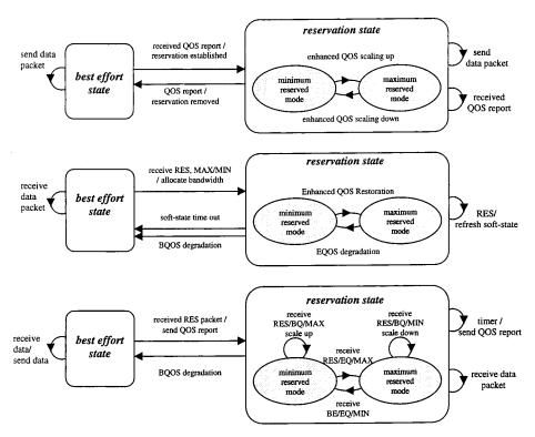
**FIG. 4.** State machine (a) a source mobile host, (b) an intermediate mobile node, and (c) a destination mobile host.
